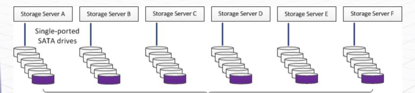
EC protection spans across servers – R6 style EC could lose two disks or two servers Allows the use of inexpensive storage server and disk architectures – maybe 1/3<sup>rd</sup> the cost
