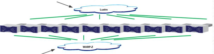
Block Layer Scale Out: Within a protection group, all disks are visible to all SSU controllers
